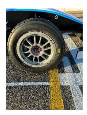
8.6.2 lateral: any wheel is beyond the grid mark meaning wheels can be on the white line but not beyond.
